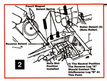
ing. Apply Mopar Gasket Maker, P/N 4318083, and install the gearshift housing using new bolts. Note the position of the shouldered pilot-bolt locations (Refer to Figure 1). Torque the six bolts to 28 N·m (21 ft/lbs.).
