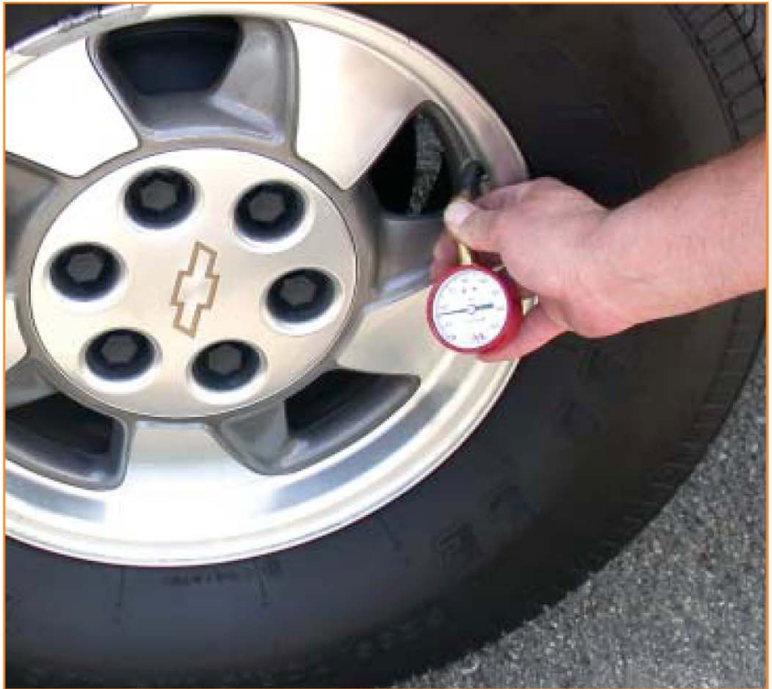
A three pound difference in air pressure between the tires can set a code.
