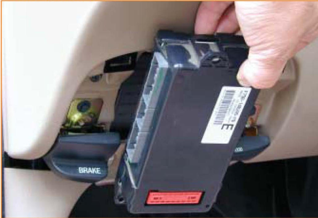
Ford uses a GEM module to control many body functions including the transfer case.
